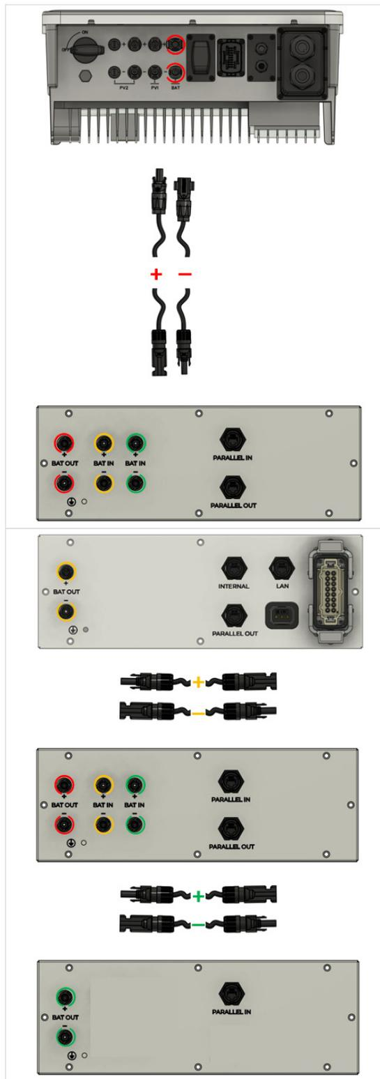
The diagram illustrates the electrical installation of three battery cabinets connected to a converter. It shows the converter's terminal block with PV2, PV1, and BAT terminals. The battery cabinets have BAT OUT, BAT IN, and PARALLEL IN/OUT terminals. The connections are as follows:
